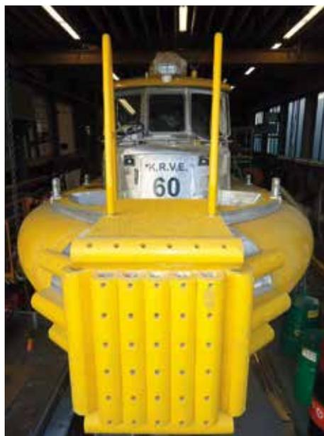
New fendersystem for the fast crew tender KRVE 60 vessel by Poly Marine Fender Systems.
